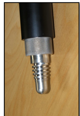
Precision Threaded Pin Screwed Into 35" Long 1.25" OD Tube
