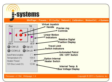
The linear scales with magenta pointers provide a visual indication of movement direction as well as relative location. A digital display below each scale shows relative pan-tilt positions in degrees.
